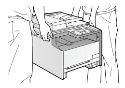
4 Put the machine down carefully at the new installation site.
